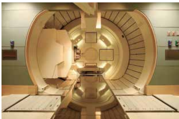
The gantry rotates and directs the protons to the patient's tumor. Photo courtesy of MD Anderson Proton Therapy Center
